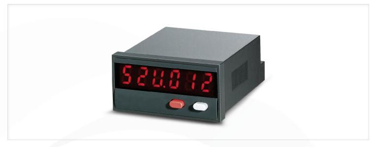
The 52UK.2 is a voltage-powered dual function counter with 4 functions in one device: counter with 2 totalizing ranges; totalizer and timer; totalizer and frequency meter; timer with 2 time ranges. For fast and slow count pulses, with 6-digit LED display for NPN, PNP input signals.
